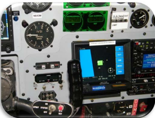
Repositioned Wingman spray guidance display screen
