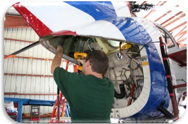
Peter Brake installs an improved turbine engine heat shield blanket on an MD 500 Helicopter
