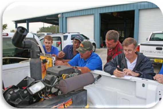
Operations staff clean and calibrate adulticiding equipment
