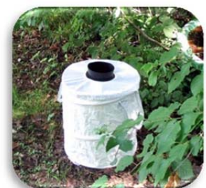
BG-Sentinel trap is used to survey for Aedes aegypti
